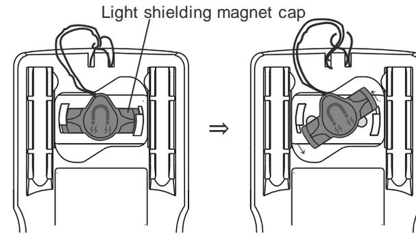
Turn the light shielding magnet cap counterclockwise to detach.
