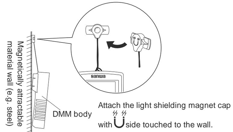
Attach the light shielding magnet cap with U side touched to the wall.
