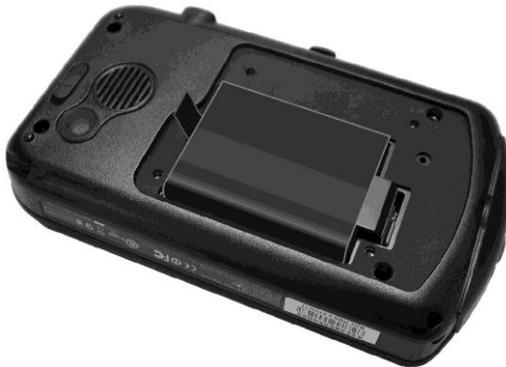
3. Replace the battery cover and tighten the four screws.
