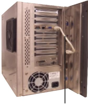
Connect PS/2 Touchpad/Keyboard cable to CPU card
