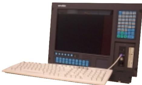
**Figure 2-9: Connect front keyboard**
