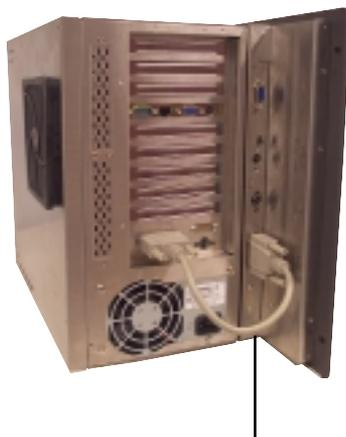
Connect USB/Indicator/Power cable to chassis
