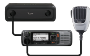
Detached Controller* Optional RMK-5 and separation cable required.
