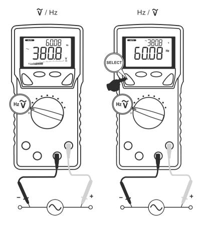
Hz input sensitivity varies automatically with a selected voltage range. 9.999V range has the highest sensitivity and the 999.9V range has the lowest. Auto ranging measurements normally set the most appropriate trigger level. You can also press the RANGE HOLD button to select another trigger level (voltage range) manually.
