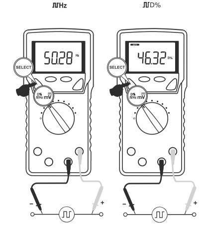
The display style of [m v̄ /m v̄], [ MHz], and [ND%] does not show the bar graph.
