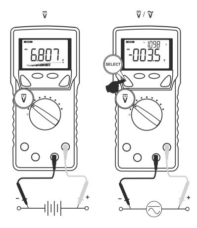
• The display style of  $[\overline{v} / \widetilde{v}]$  does not show the bar graph.
