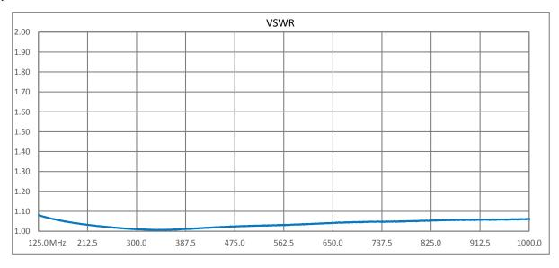
Click the following link (or enter part number in "SEARCH" on website) to obtain additional part information including price, inventory and certifications: Type N M/F Bulkhead Coaxial RF Surge Protector, 125MHz - 1GHz, DC Block, 500W, 800uJ, 50kA, Blocking Cap, Hole Mount IS-B50HN-C2-MA
