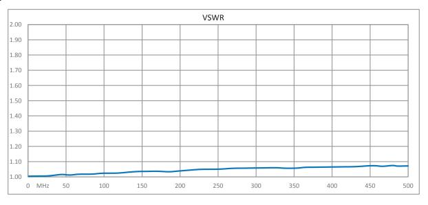
Click the following link (or enter part number in "SEARCH" on website) to obtain additional part information including price, inventory and certifications: Type N M/F Coaxial RF Surge Protector, 1.5MHz - 700MHz, DC Block, 500W, 20mJ, 50kA, Blocking Cap, Bracket Up, Hole Mount IS-B50HN-C0-MA
