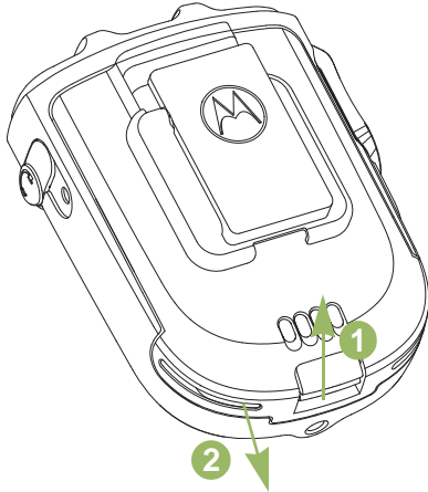
Figure 2.3: Removing the battery from the WRSM
