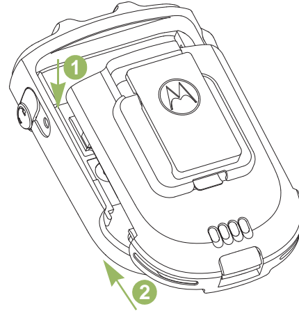
Figure 2.2: Attaching the battery into the WRSM
