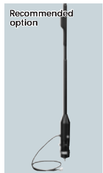
AT230 AUTOMATIC TUNING ANTENNA (Moonraker Australia Pty. Limited) 2.6m (8.5ft) length mobile mount whip antenna covers 2-30MHz with automatic tuning function. Continuous CW transmission at high power not guaranteed with AT230.
