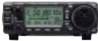
To extend battery life, the back lighting for the display and buttons automatically turns off when unused.
