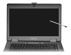
Use the included stylus to select objects on the screen. The stylus can be stretched for better grip and handling.
