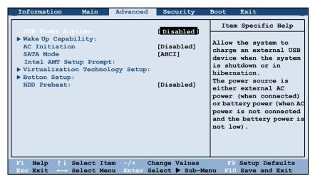
**USB Power Anytime** allows the system to charge an external USB device when the system is shutdown or in hibernation. The power source is either external AC power (when connected) or battery power (when AC power is not connected and the battery power is not low).
