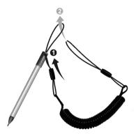
2. Insert the other loop end to the tether hole on the computer (as indicated by • below). Then, insert the stylus end through the loop (as indicated by @ below) and pull it tight.
