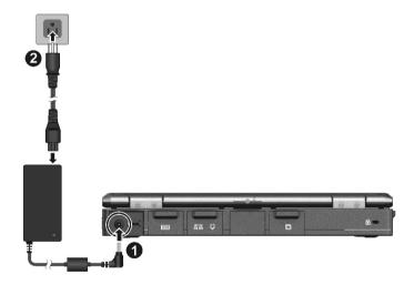
3. When the AC adapter is connected, power is being supplied from the electrical outlet to the AC adapter and onto your computer. Now, you are ready to turn on the computer.
