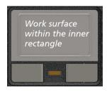
The touchpad consists of a rectangular pad (work surface) and a left and right buttons. To use the touchpad, place your forefinger or thumb on the pad. The rectangular pad acts like a miniature duplicate of your display. As you slide your fingertip across the pad, the pointer (also called cursor) on the screen moves accordingly. When your finger reaches the edge of the pad. simply relocate yourself by lifting the finger and placing it on the other side of the pad.
