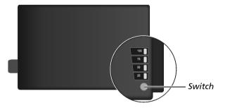
The value of the corresponding green segment indicates the relative percentage of the battery charge. The battery pack is fully discharged when you see no segment glowing green.
