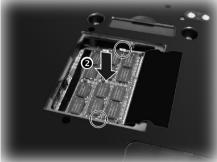
**CAUTION:** If the RAM module is difficult to insert or difficult to push down, do not force it. Check once more to ensure that the module is positioned correctly.
