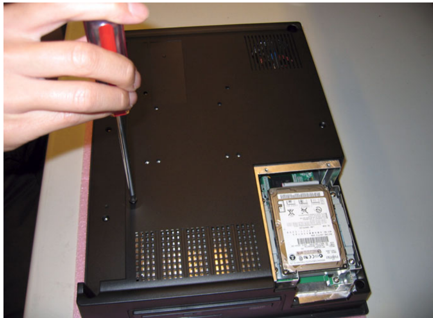
Figure A.2 Unfastening the rear cover
