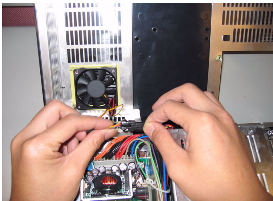
Figure A.3 Disconnecting the fan connector
