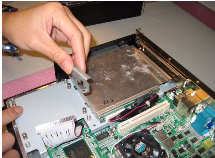
Figure A.14 Removing the fixed brace
