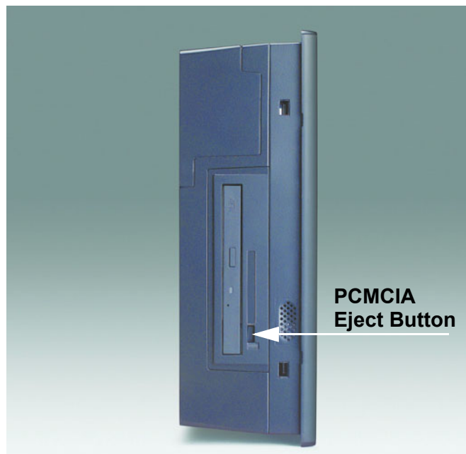
Figure 3.2 Inserting and ejecting a PCMCIA card
