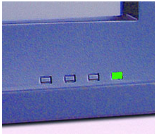
Figure 3.5 LED & light sensor
