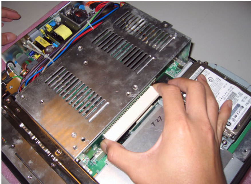
Figure A.5 Removing the PCI riser card
