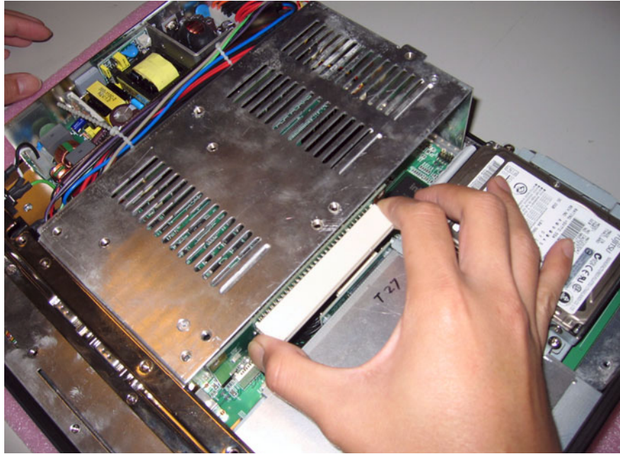
Figure 3.3 PCI bus expansion
