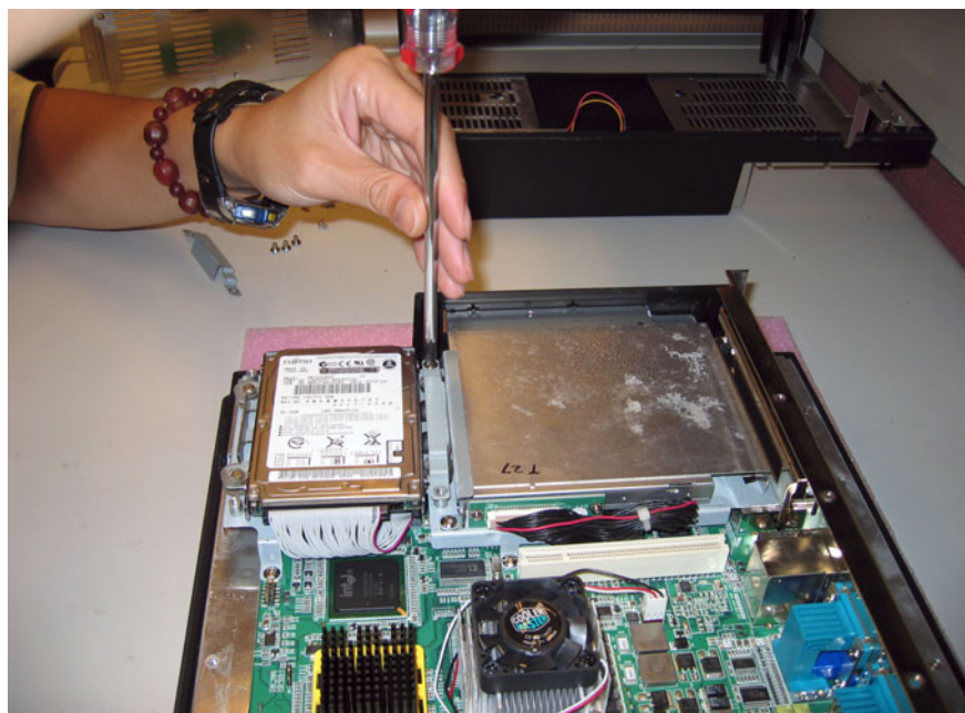
Figure 4.7 Aligning the HDD frame
