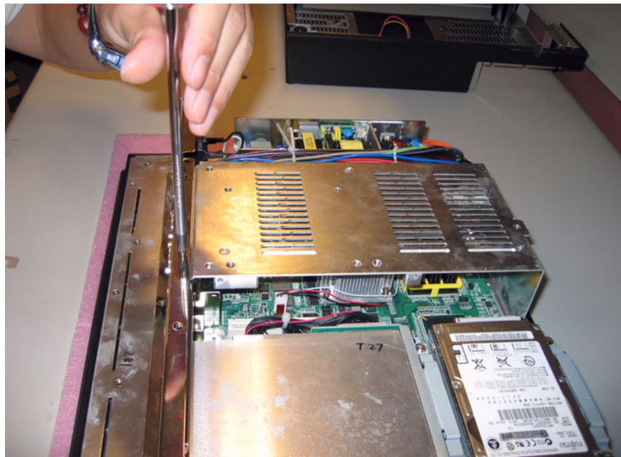
Figure A.6 Unfastening the middle plate
