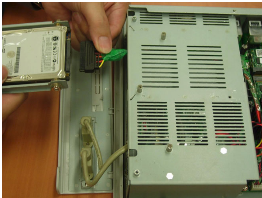
Figure 4.7 Plugging in the SATA Cable
