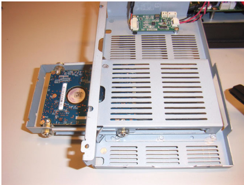
Figure 4.8 Fastening the HDD metal frame to the HDD
