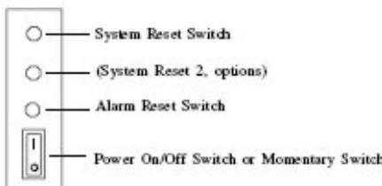
**System Reset 1:** Press this switch to reinitialize the system. This is the same as the hardware reset button. (Default setting)
