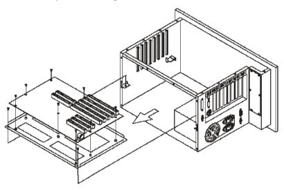
Figure 4-1: Detaching the backplane and bracket
