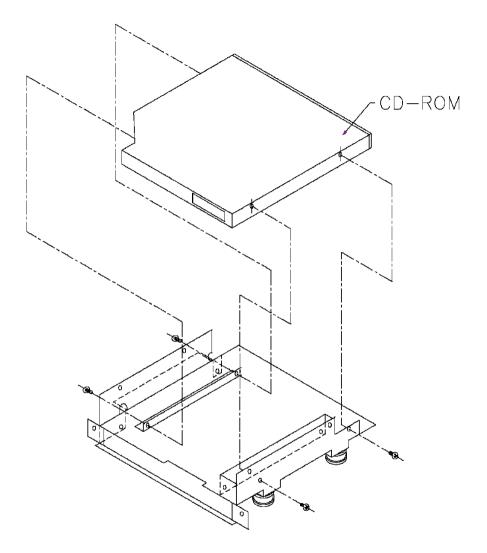
Figure 2-7: Installing a CD-ROM
