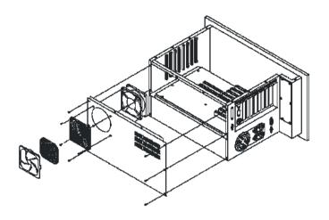
Figure 2-2: Opening the rear panel
