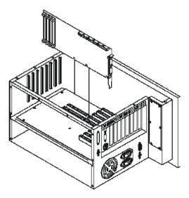
Figure 2-3: Installing add-on cards
