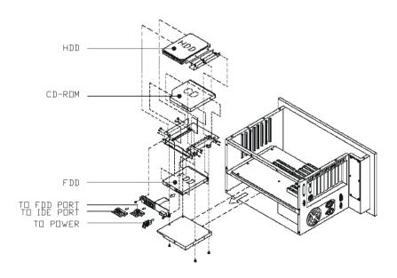
Figure 2-4: Installing optional disk drives - overall view
