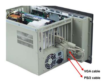
Figure 2-8 Connecting cables
