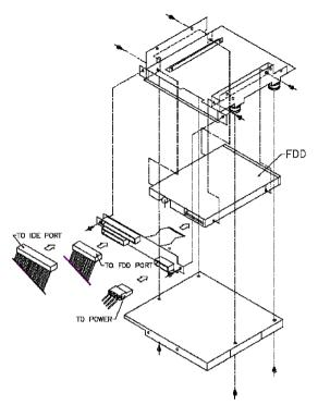
Figure 2-5: Installing an FDD
