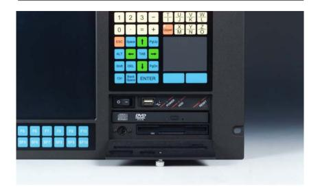
Figure 1-4: Front control panel
