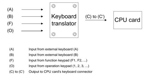
Figure 4-4: Keyboard translator input/output (basic schematic)
