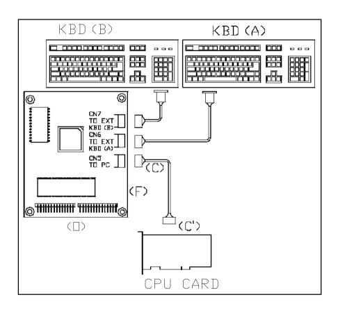
Figure 4-5: Keyboard translator input/output (detailed schematic)
