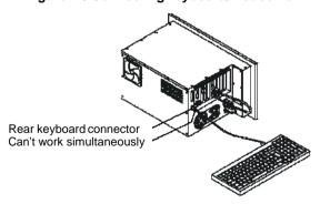
Figure 2-10 Connecting keyboard from back chassis
