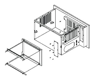
Figure 4-3: Installing the LCD backlight
