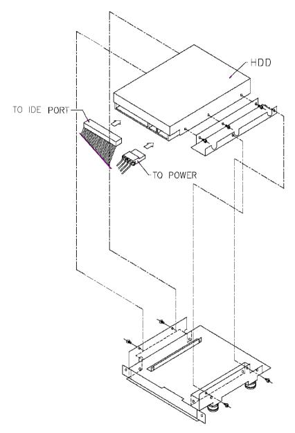
Figure 2-6: Installing an HDD
